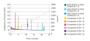
Temperature: 50°C; stroke: 1 mm; frequency: 50 Hz; test ball: SUJ-2; test disk: SUJ-2, procedure A
