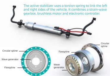
The strain-wave gear set provides repeatable accuracy for positioning inertial loads with high torque. It consists of a circular spline ring gear, a flexspline cup and an elliptical-shaped wave generator that is slightly smaller than the flexible ring and has two fewer teeth. The flexspline deforms to the shape of the wave generator and works independent of the shaft. The flexspline rotates much slower than the wave generator and in the opposite direction.
